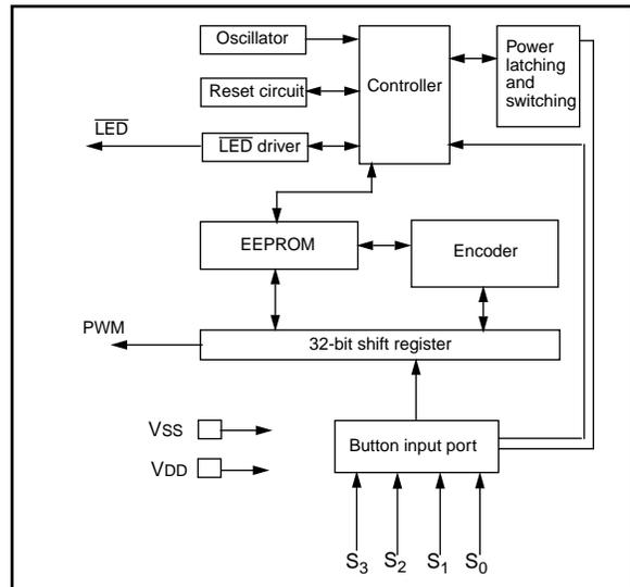
The HCS301 combines a 32-bit hopping code generated by a non-linear encryption algorithm, with a 28-bit serial number and six status bits to create a 66-bit transmission stream. The length of the transmission eliminates the threat of code scanning and the code hopping mechanism makes each transmission unique, thus rendering code capture and resend (code grabbing) schemes useless.
