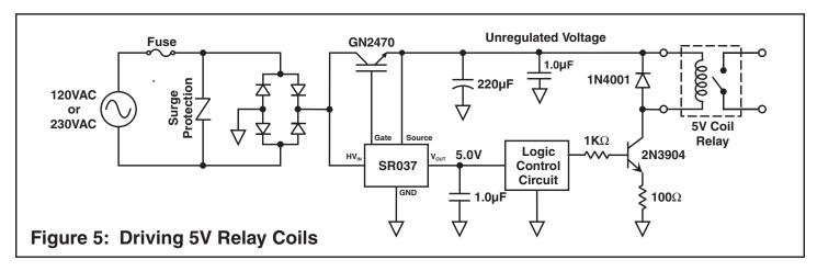
The circuit shown in Figure 5 uses the SR037 to supply a regulated 5.0V for the logic control circuitry while the unregulated voltage is used to drive a 5.0V coil relay. To overcome the voltage variation of the unregulated line, a bipolar transistor is used to
