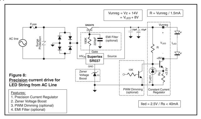
The circuit uses the SR037or SR036 and GN2470 to drive a string of LEDs from AC power line.
