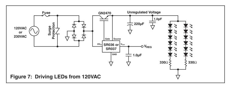
The circuit shown in Figure 7 uses the SR036 or SR037 to drive 12 high efficiency red LEDs from an AC line. The average LED current is approximately 20mA.
