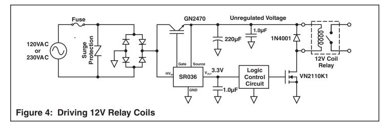
The circuit shown in Figure 4 uses the SR036 to supply a regulated 3.3V for the logic control circuitry while the unregulated voltage is used to drive a 12V relay coil. The operating voltage for a 12V relay coil is typically very wide and can therefore operate directly from the unregulated line.
