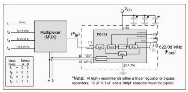
All components outside the dotted line box are user supplied components. This is just one possible configuration of the FX-104. For additional information about your specific needs, please contact our factory.
