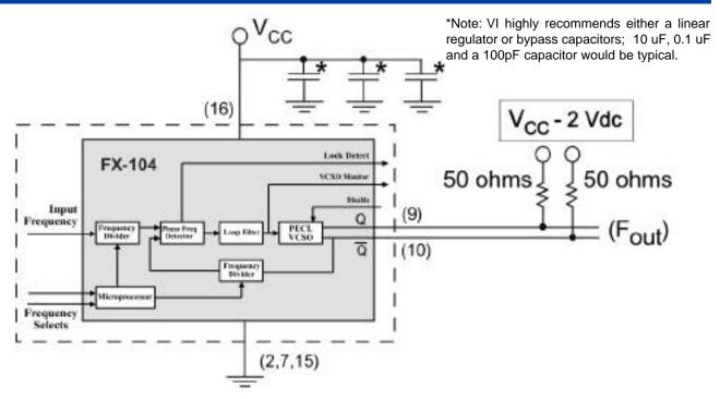
All components outside the dotted line box are user supplied components and/or connections. This is just one possible configuration of the FX-104. For additional information about your specific needs please contact our Factory.
